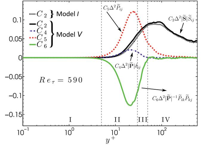
Fig. 4. Coefficients for SGS model for Models I and V.
