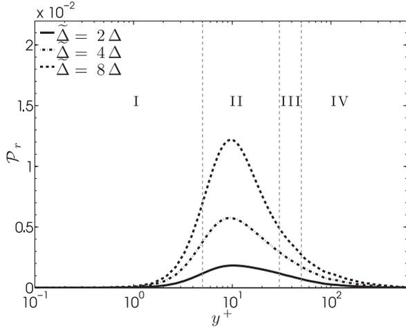
Fig. 2. Profile of  $P_r$  across the channel half-width at  $Re_\tau = 590$ .
