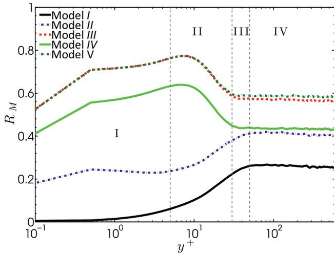
Fig. 3. Correlation coefficient,  $R_M$ , applied to Models I to V at  $Re_\tau = 590$ .
