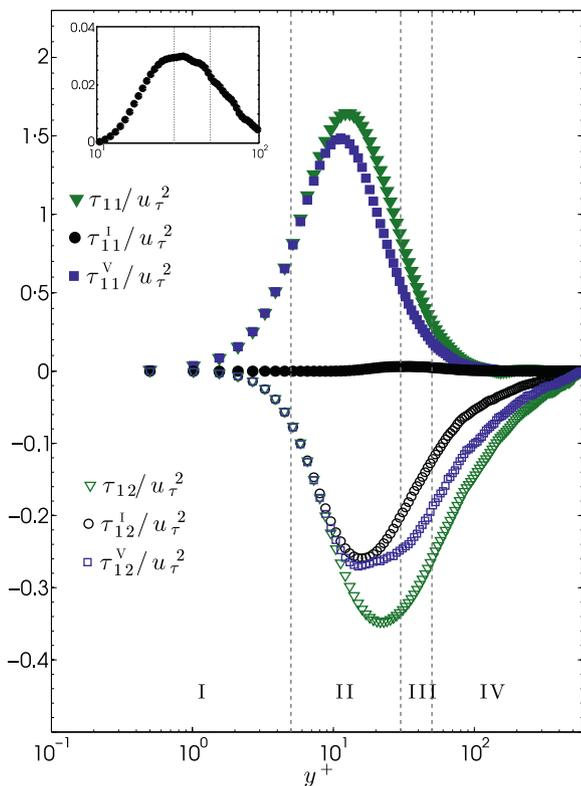
Fig. 5. Modeled and exact components of SGS stress tensor by applying Model I and Model V.
